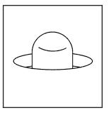
Your vehicle has a light sensor located on top of the instrument panel. Make sure it is not covered, or the headlamps will be on when you don't need them.
